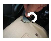
(4) Rotate the hook into position as shown.
