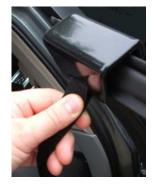
(5) Place the large black hook at the other end of the strap over the car door window frame as shown.
