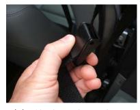
(6) Lift the tab on the adjustment buckle to change the length of the strap, and relock to secure the strap.
