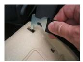
(2) Position the silver ramp hook over the long slot at the unsupported corner of the ramp. (the other corner rests on the car seat)
